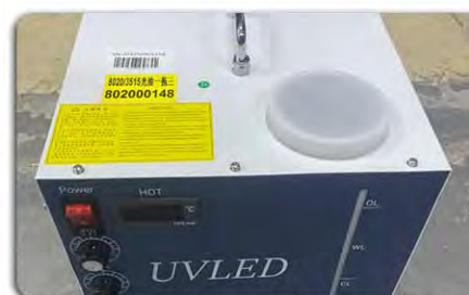
High-power water-cooled UV lamp for long service life.
