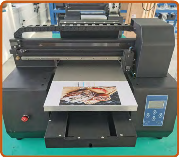
1. The vacuum printing platform can be raised and lowered by 12cm, and a cylindrical fixture can be added
