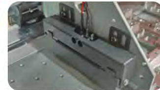
Anti-collision device. To prevent the print head from being scratched or hit
