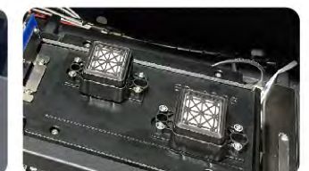
Elevation Capping Station
