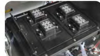
Aluminum capping station. The rise and fall are smooth and not wobbly
