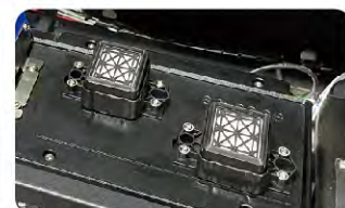
Elevation Capping Station
