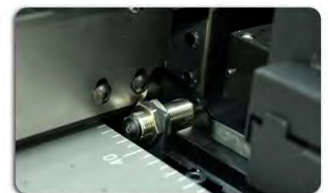
Infrared height detection to prevent printhead contact (14cm lift).
